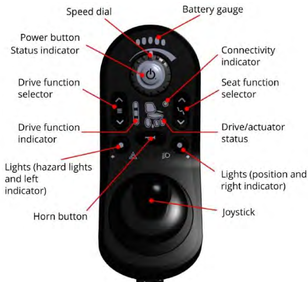
Control Panel with No Tilt & Lighting System
