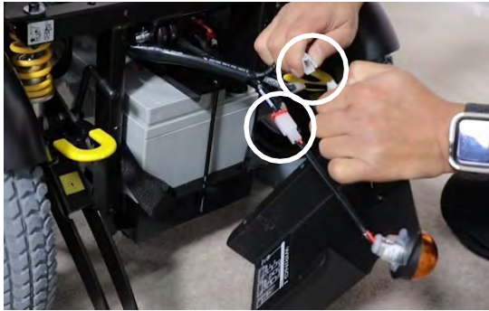
step 8. Disconnect the two light cables
