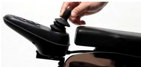
Pull the joystick towards the user
