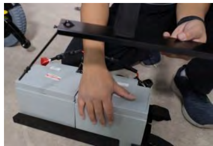
step10. Use 8mm open wrench to loosen up this bolt.
