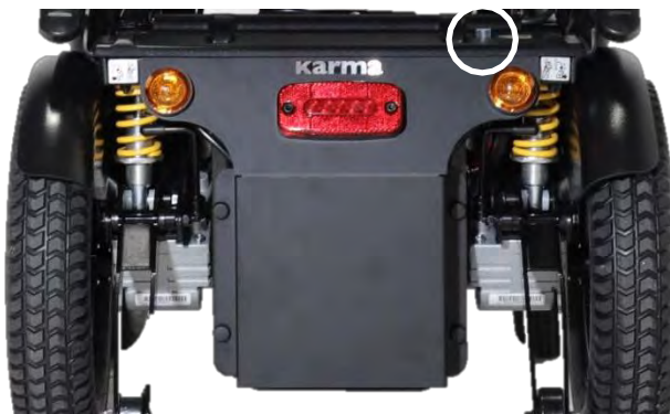
Circuit breaker location
