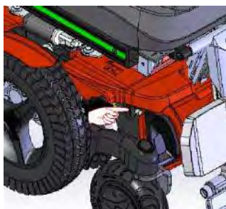
Position of the circuit breaker
