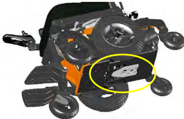
MID chassis with Dahl Docking plate mounted.
