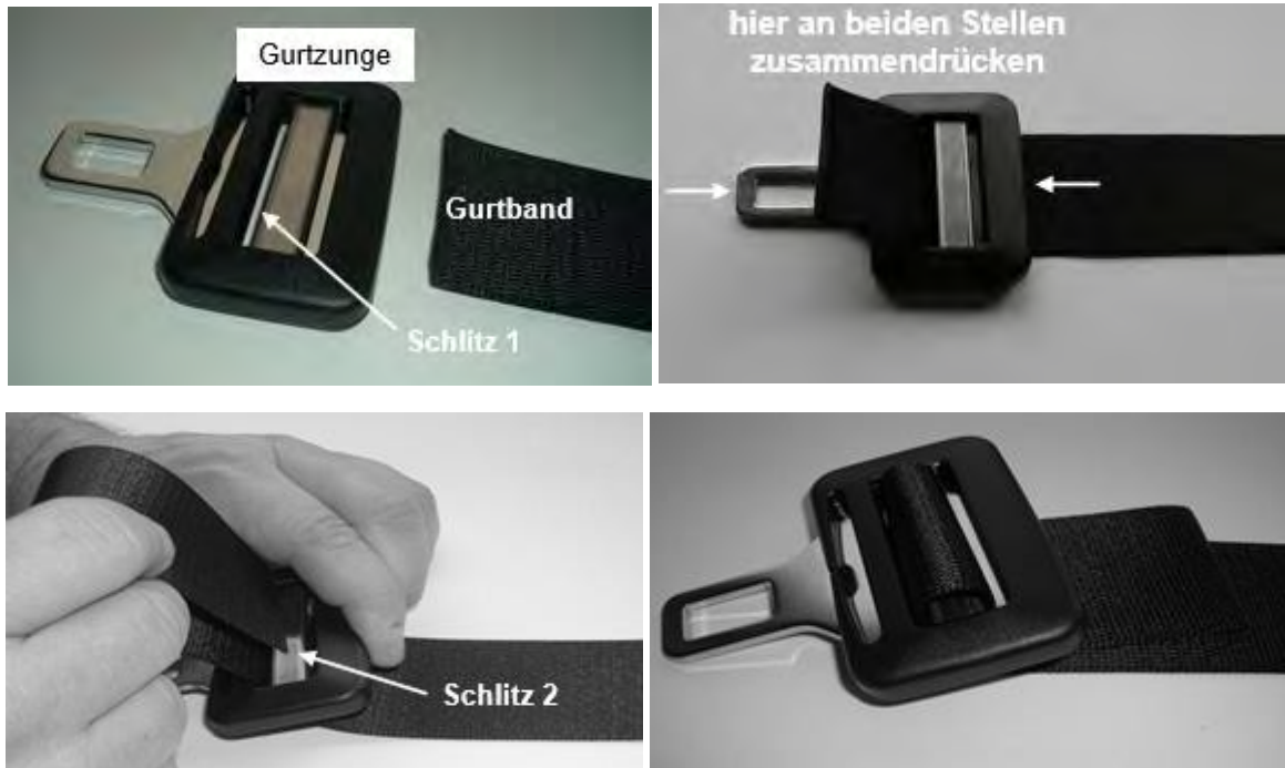
Figure 2: Procedure for looping in the webbing
