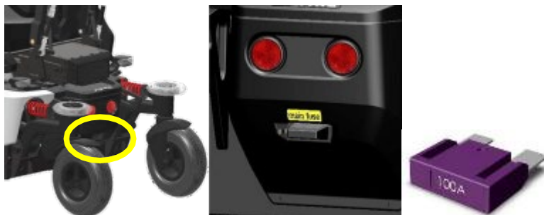
Position fusible principal Fusible principal
