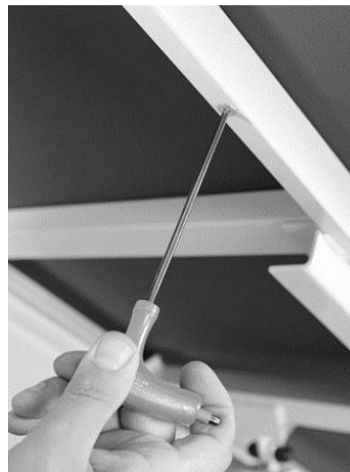
Figure 2: Unscrewing the lying surface
