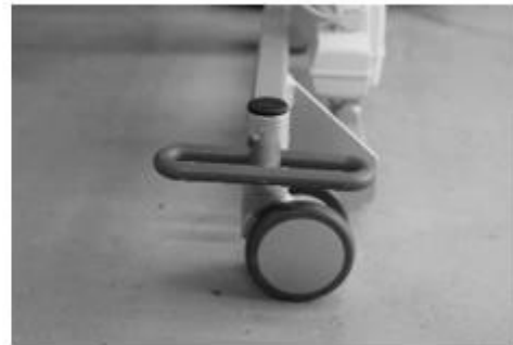
Figure 7: Castors in braked and unbraked condition
