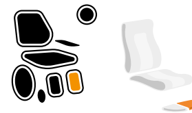
Figure 5.22. Symbol for adjusting the length of length compensatory leg supports.
