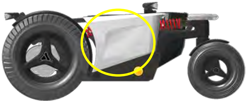
The battery box
