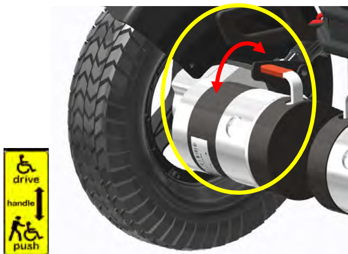
Testing the brake release
