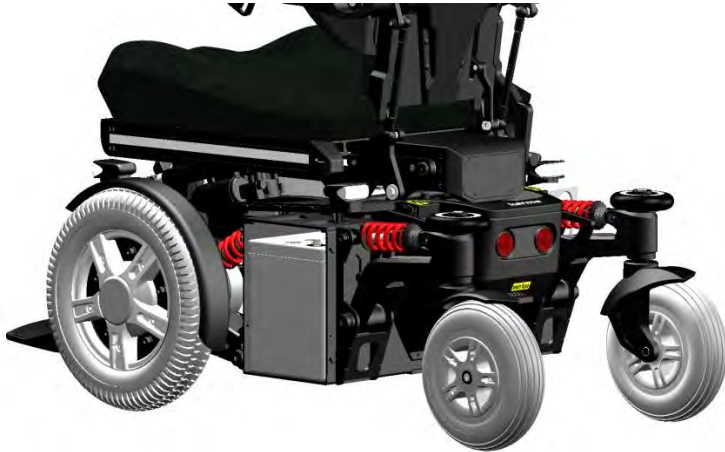
Position and access of the maintenance free batteries
